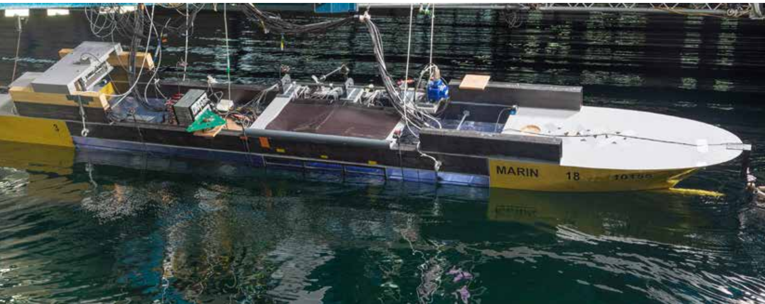
Complex flooding scenarios tested with a free floating cruise ship with a large external damage and a realistic internal compartmentation covering 6 decks
